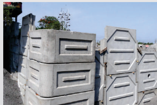
Newly developed corner unit for RSRW.
