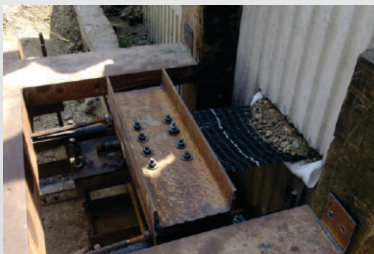
Onsite Geogrid pull-out test.
